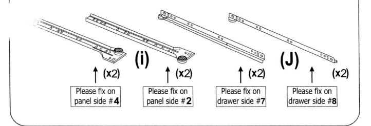
02 The wheel to the front! The wheel to the front! H PRE-DRILLED HOLES H H H H Right side (+)SPACE (+) BACK SPACE (-) BOTTOM Division / left side Qty **Drawer Runner 350mm**
